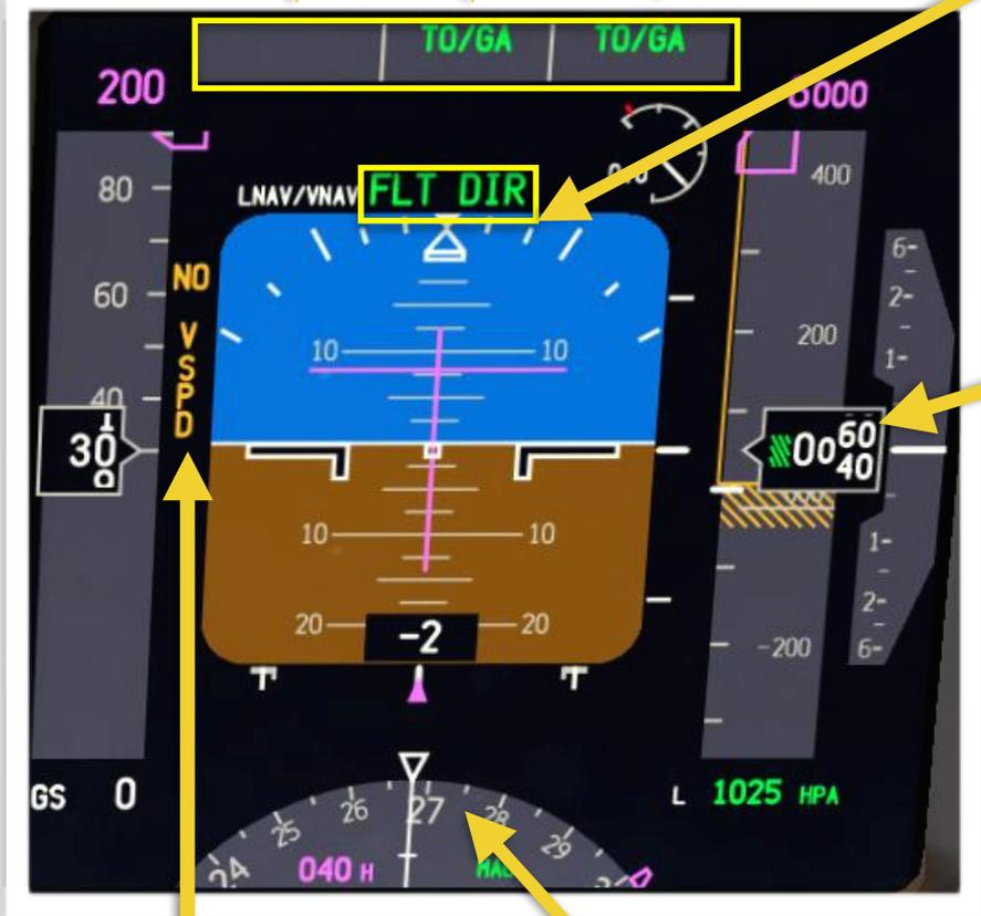
**CHECK ALTIMETERS TO BE WITHIN 75FT AIRPORT ELEVATION**
