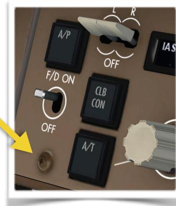
*The TOGA buttons are located just in front of the thrust levers. There is also a "ghost button" that replicates the TOGA function just below the Captain's Flight Director switch (with the shape of a screw). However it is highly recommended to assign a key or a button on your joystick to quickly use this function.*
